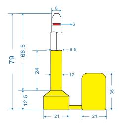
The pin diameter is 9.5mm It is suitable to the old standard container also
