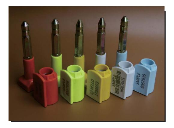
The bolt seals complies with ISO17712,To avoid opening it with rotating method. The new structure has metal antispin design. if so, It only can be opened by cutting or loading. The tensile strength is more than 1850kgs.
